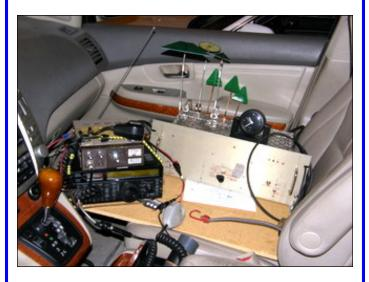
And thanks to **Rick K1DS** for assembling the antennas. I used a 2-position coax switch to route the 2-Meter signal to an antenna, or to the xvtr IF input/output. So all I had to do for microwave use was throw the coax switch, and select desired band on front panel. **A really neat job, Randy.**
